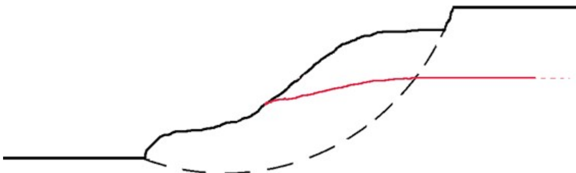
Pullout of the reinforcement behind the slip surface - type of failure 2
