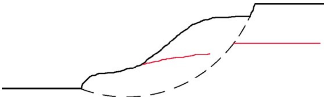
Breaking of reinforcement - type of failure 1
