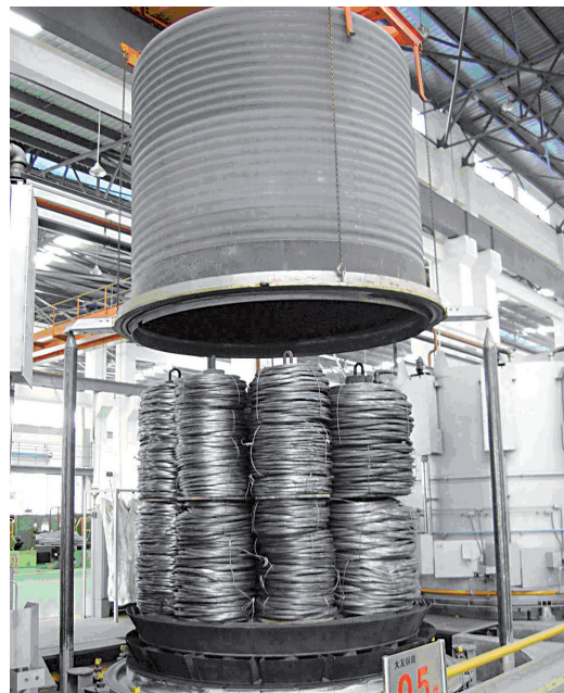
Fig. 4 6 — Retort being lowered into position.
