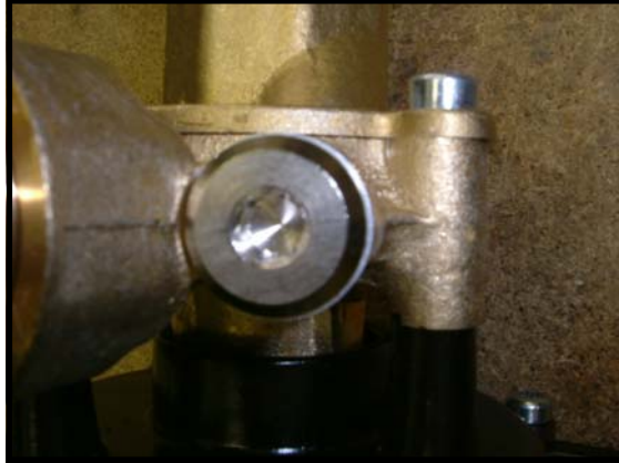
Figure 16. Priming Screw
