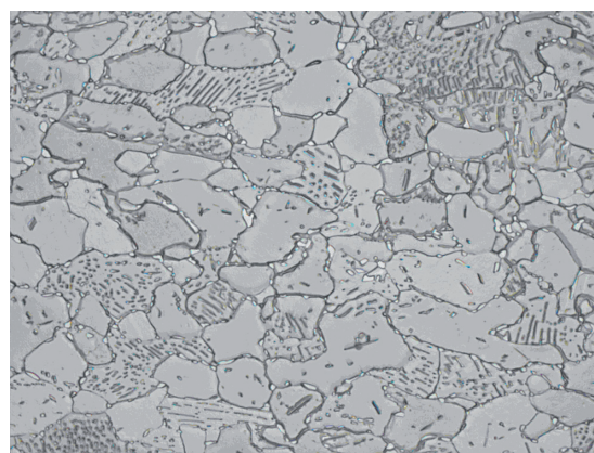
Fig. 8 7 — Process annealed microstructure – low-carbon alloy steel (photomicrograph courtesy of Aston Metallurgical Services Co., Inc.).
