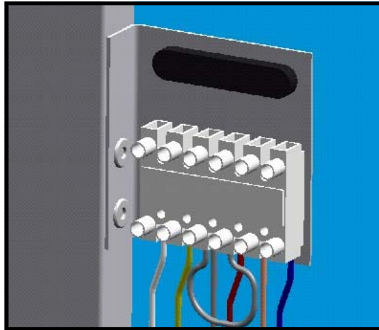
Figure 12 Alarm Terminal Location
