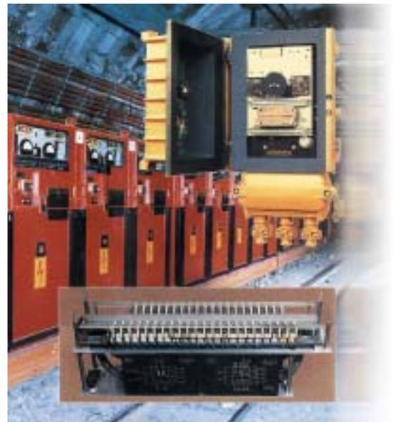
High-voltage Ground Fault Monitor 1976
