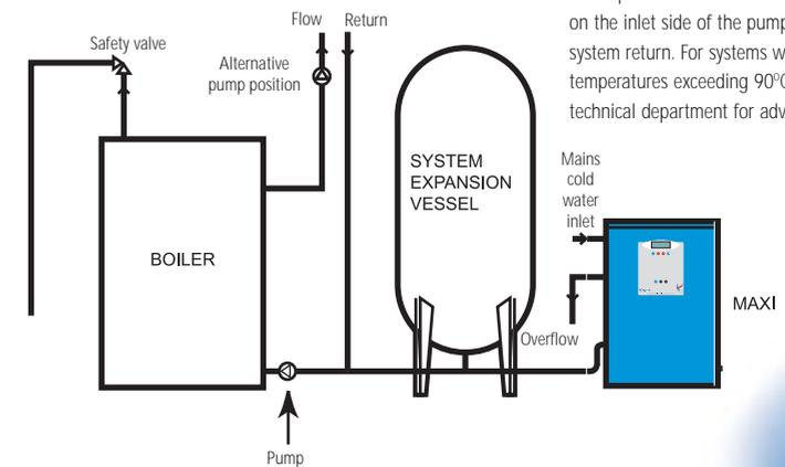
The expansion vessel is usually connected on the inlet side of the pump on the system return. For systems with flow temperatures exceeding 90°C contact our technical department for advice.
