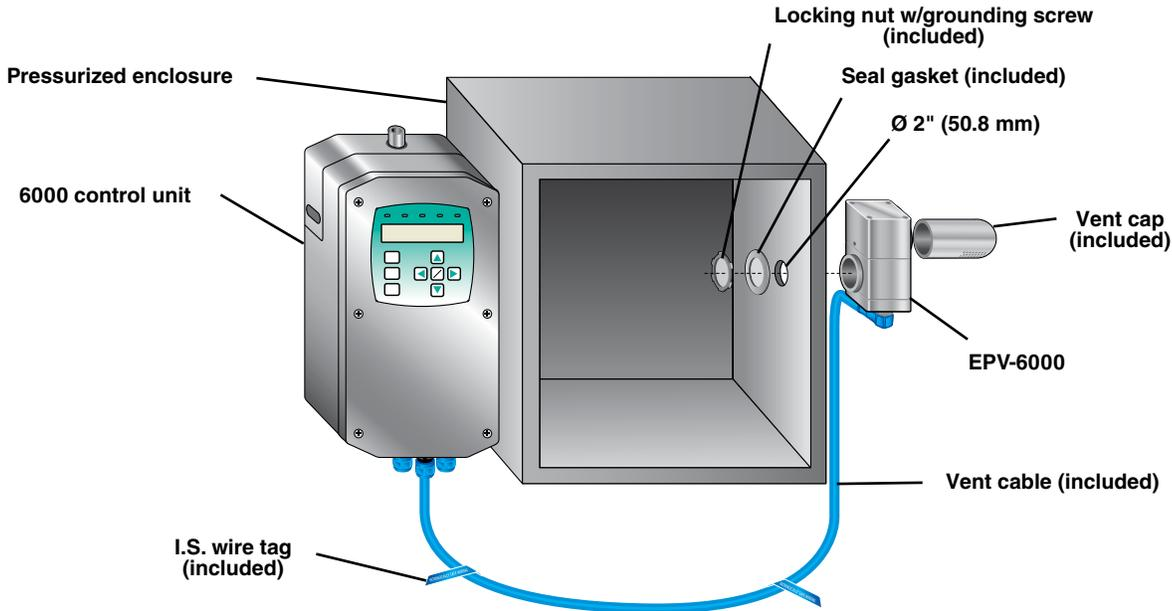
**Vent mounted on the inside of the enclosure**
