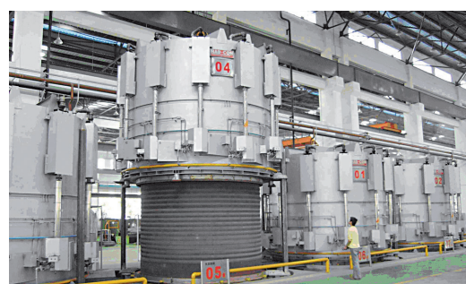
Fig. 5 6 — Heating bell being lowered in place.
