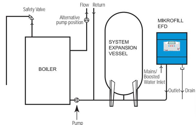
The expansion vessel is usually connected on the inlet side of the pump on the system return. For systems with flow temperatures exceeding 90°C contact our technical department for advice.
