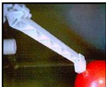
Figure 15 Float Adjustment
