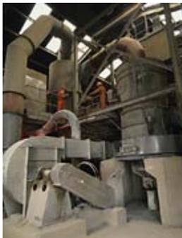
Dust explosion events have been recorded in industrial facilities, particularly within the food industry, for over 200 years. Processes such as milling, grinding, drying or even conveyance and storage of combustible grains and powders have the possibility for dust to be released into the atmosphere and as a result have the potential to produce dust explosion events.
