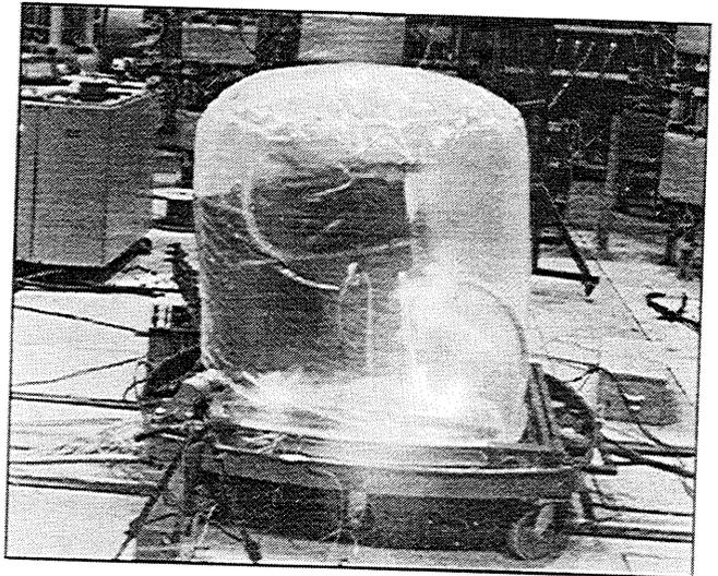
**Figure 2** Time lapse photograph of a 0.3m<sup>3</sup> enclosure under arcing conditions. Photograph shows gas curtain exploding, while large amounts of sparks are emitted from the bottom edge of the enclosure door panel.
