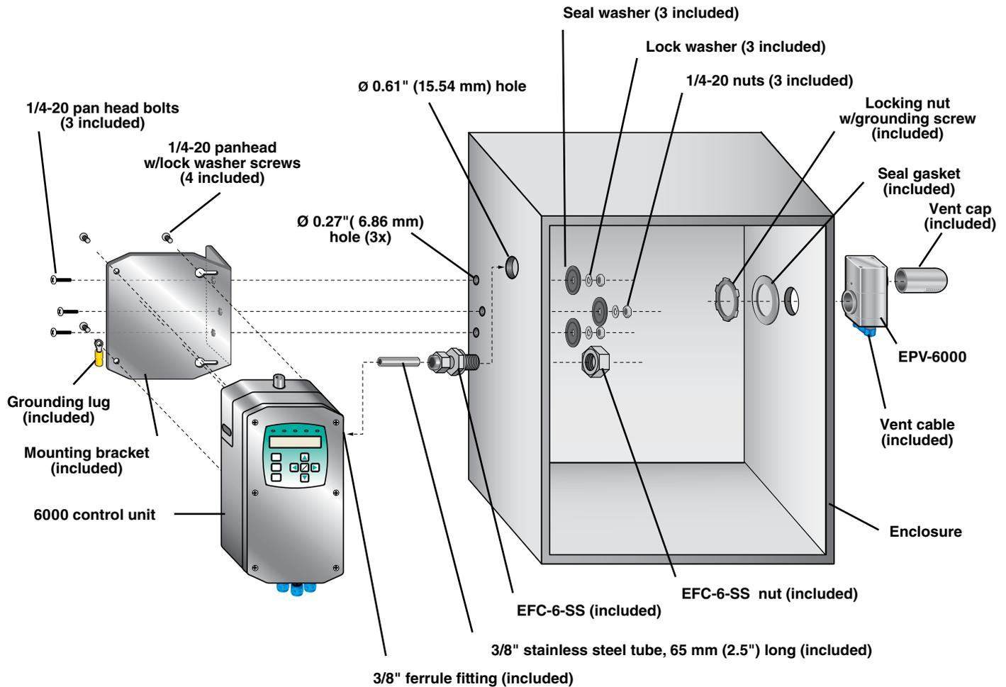
1. Drill holes using template. Check the scale if printing an electronic version.
