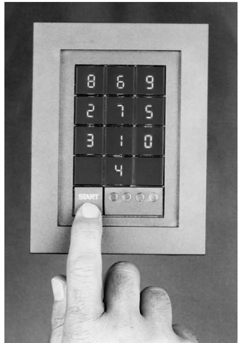
Figure 5.26 Hirsch ScramblePad™ Secure Electronic Digital Keypad. The ScramblePad is also available with the dual technology of a hidden proximity card reader located behind the keypad; and for even higher security applications, a combination of biometrics (fingerprint) with a smart card (fingerprint storage) to activate the ScramblePad. Courtesy of Hirsch Electronics Corporation, Irvine, CA.
